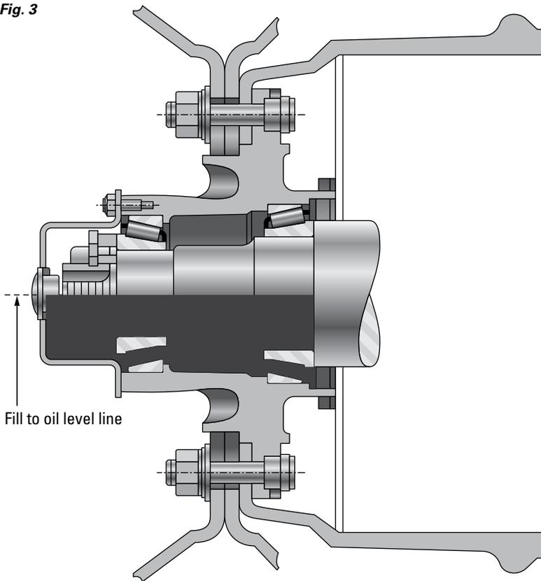
With the axle on a level surface, fill housing with oil to bottom of the fill plug
