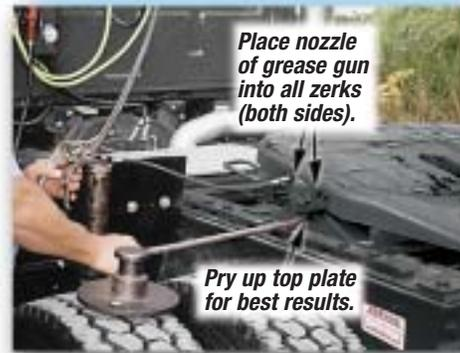
*Place nozzle of grease gun into all zerks (both sides).*
