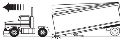
**WARNING** Failure to properly install, operate, or maintain this fifth wheel could result in tractor and trailer separation causing death or serious injury to others.
